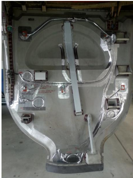
Figure 4: FTI on left hand MLG door (left) and VG's installed on MLG door (right) on DLR ATRA A320. Courtesy of DLR.
