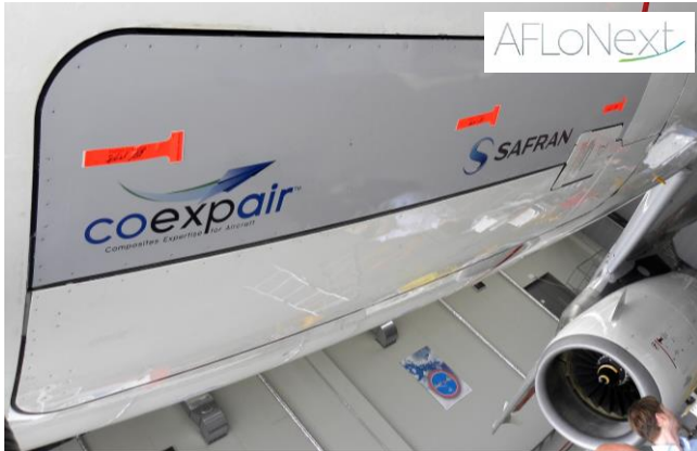
Figure 16: Successful functional test of the 2nd NLGD (flying part) performed at DLR August 1, 2017.
