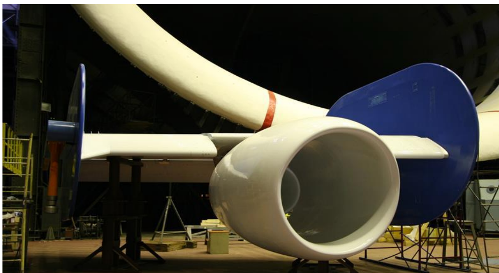
Figure 4: Wind tunnel model of generic wing/pylon/engine wing section prepared for testing at the TsAGI T-101 wind tunnel.
