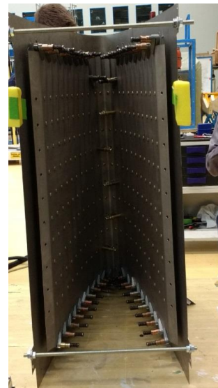
Figure 2: HLFC leading-edge demonstrator at full scale.
