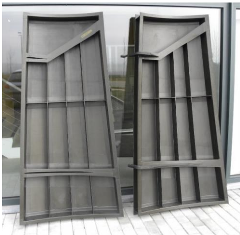
Figure 13: “I” stiffener panel doors manufactured by Coexpair & SSA in European IMS&CPS FP7 project (experience gained & manufacturing risks mitigated).
