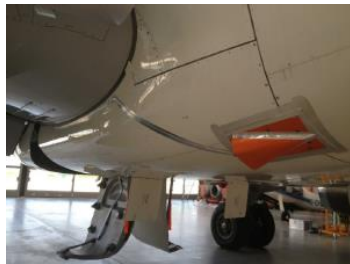
Figure 5: Camera position (top) and camera and fairing (bottom) on DLR ATRA A320. Courtesy of DLR.
