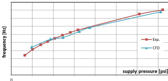
Figure 6: Comparison of the dependence of the frequency of the oscillation jet on supply pressure.
