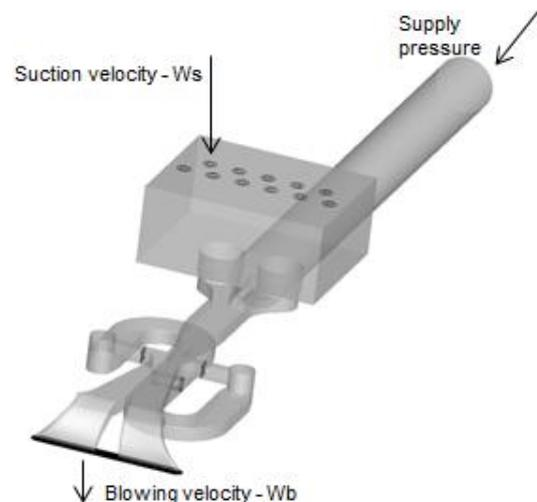
Figure 5: Isolated SaOB actuator used for CFD studies.
